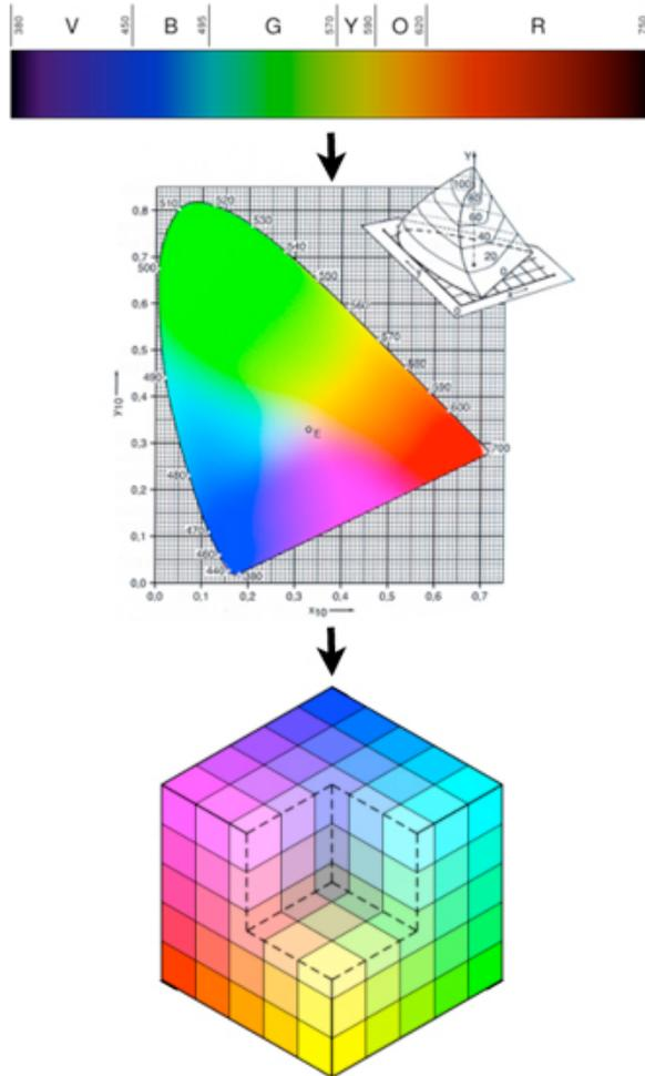
**Figure 3.** Method used to convert nm to RGB. Conversion from nm to CIE XYZ coordinates, followed by conversion from CIE XYZ coordinates to RGB coordinates.
